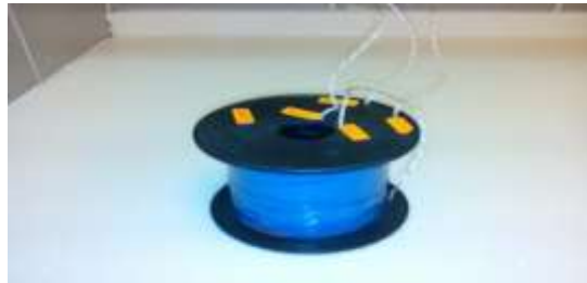
Figure 3: Bifilar Coil for Bedini SSG
