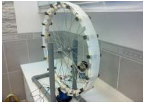
Figure 6: prototype of original Bedini SSG rotor
