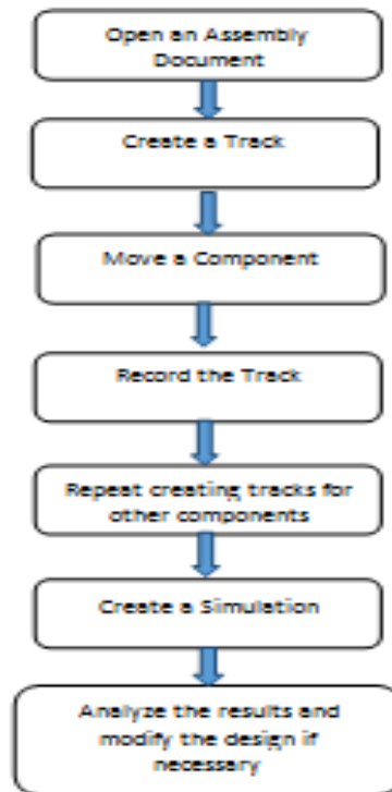
Fig 1: Flow chart for simulation
