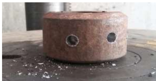
Fig. 7: Image shows drilled hole on workpiece for setup of 30° angle.
