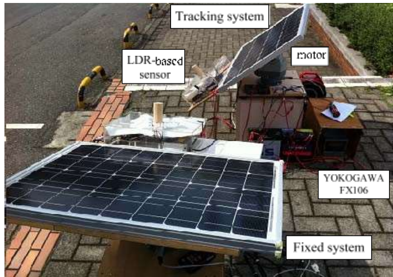
Figure 8. Actual photograph of the experimental prototype.
