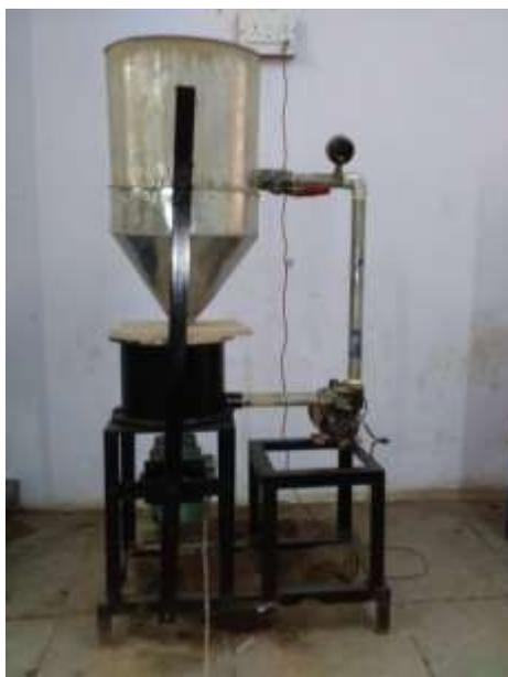
Photograph of jet erosion tester
