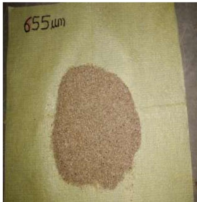
Photograph of sand particle size 655 $\mu\text{m}$
