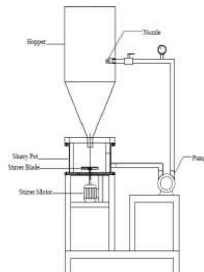
Fig.1 Schematic Diagram of Jet Erosion Tester
