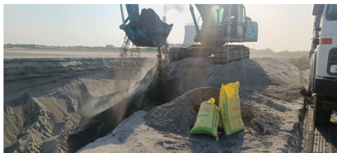
Fig. 2. Coal bottom ash (CBA) produced by Koradi Super Thermal Power Station, Koradi, Panjara, Nagpur, Maharashtra 441111
